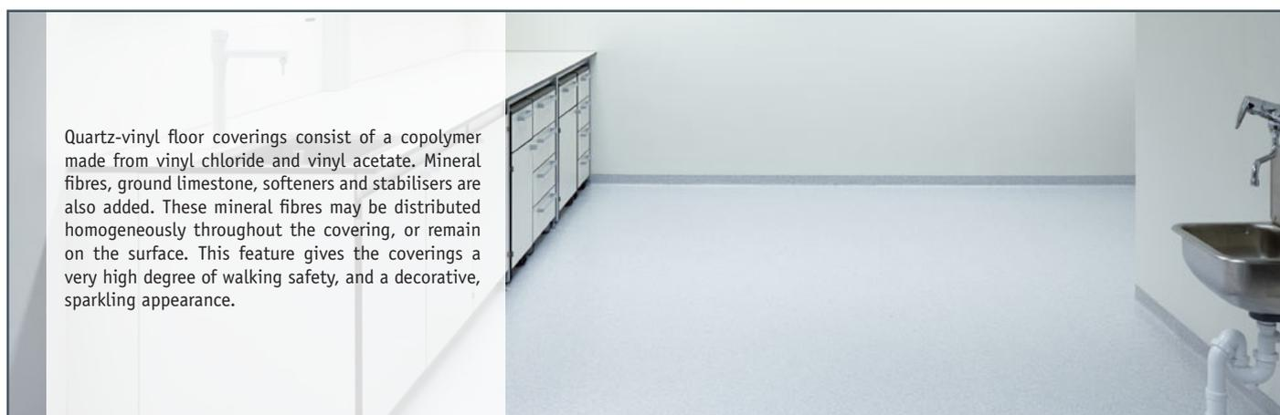
Quartz-vinyl floor coverings consist of a copolymer made from vinyl chloride and vinyl acetate. Mineral fibres, ground limestone, softeners and stabilisers are also added. These mineral fibres may be distributed homogeneously throughout the covering, or remain on the surface. This feature gives the coverings a very high degree of walking safety, and a decorative, sparkling appearance.
