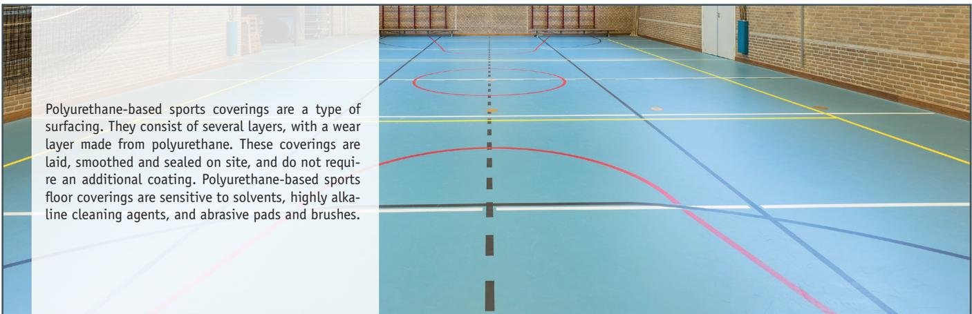
Polyurethane-based sports coverings are a type of surfacing. They consist of several layers, with a wear layer made from polyurethane. These coverings are laid, smoothed and sealed on site, and do not require an additional coating. Polyurethane-based sports floor coverings are sensitive to solvents, highly alkaline cleaning agents, and abrasive pads and brushes.
