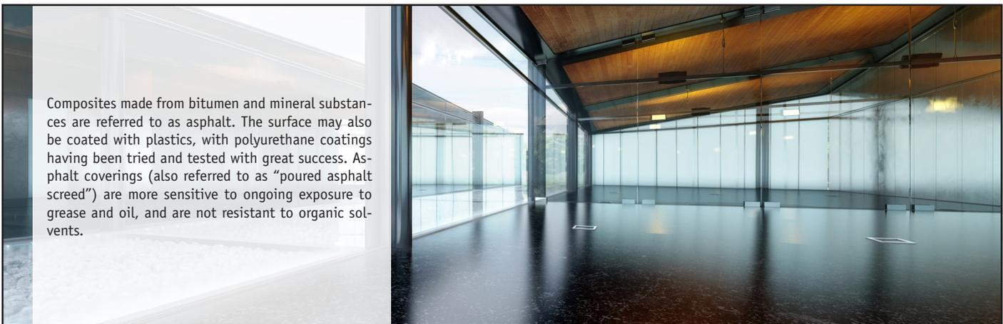
Composites made from bitumen and mineral substances are referred to as asphalt. The surface may also be coated with plastics, with polyurethane coatings having been tried and tested with great success. Asphalt coverings (also referred to as "poured asphalt screed") are more sensitive to ongoing exposure to grease and oil, and are not resistant to organic solvents.
